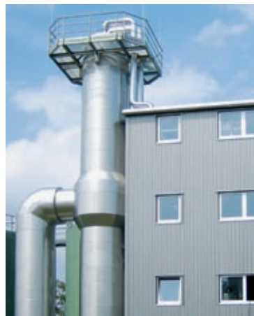
Falling film forced circulation evaporation plant with mechanical vapour recompression. Evaporation rate: 9,000 kg/h
