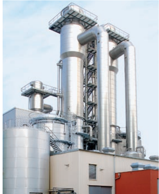
Concentration of potato juice Two pre-evaporators with mechanical vapour recompression and a finisher with thermal vapour recompression. Evaporation rate in total: 152,000 kg/h
