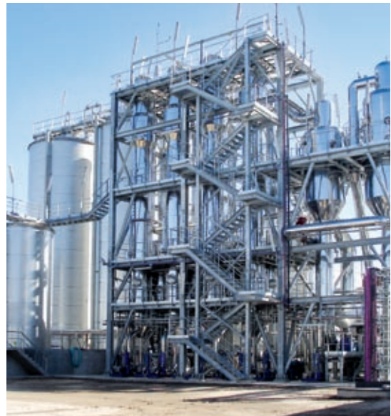
Six-effect falling film forced circulation evaporation plant. Evaporation rate 31,000 kg/h
