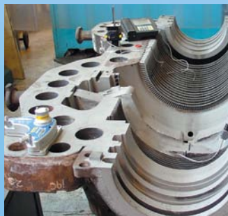
Geometric alignment (surface profile, bearing shells, bores)
