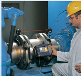
Laser shaft alignment (horizontal, vertical, machine trains)
