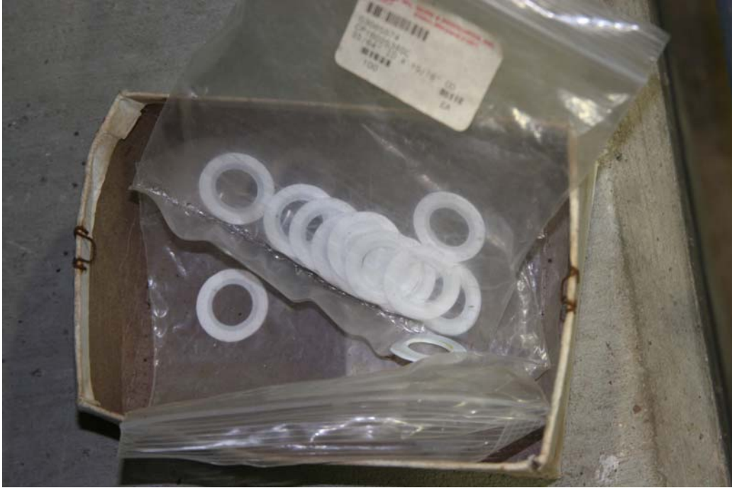
Top photograph, chlorine container gaskets. Bottom, we often take our students on a walking tours of a large chlorine facilities.
