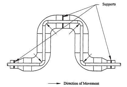
Figure 8-2. Double Containment Piping Expansion Loop Configuration (Source: SAIC, 1998)
