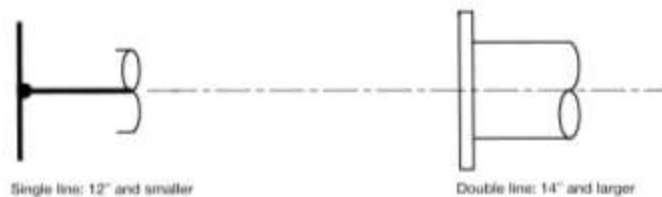
Figure 4-14. Slip-on flange drawing symbols.
