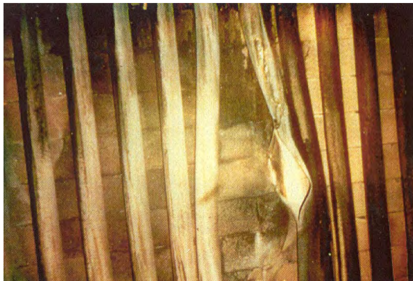
Figure 3-8. Failed Boiler Tube
