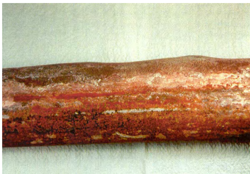
Figure 3-7. Metal Fatigue on Boiler Tube
