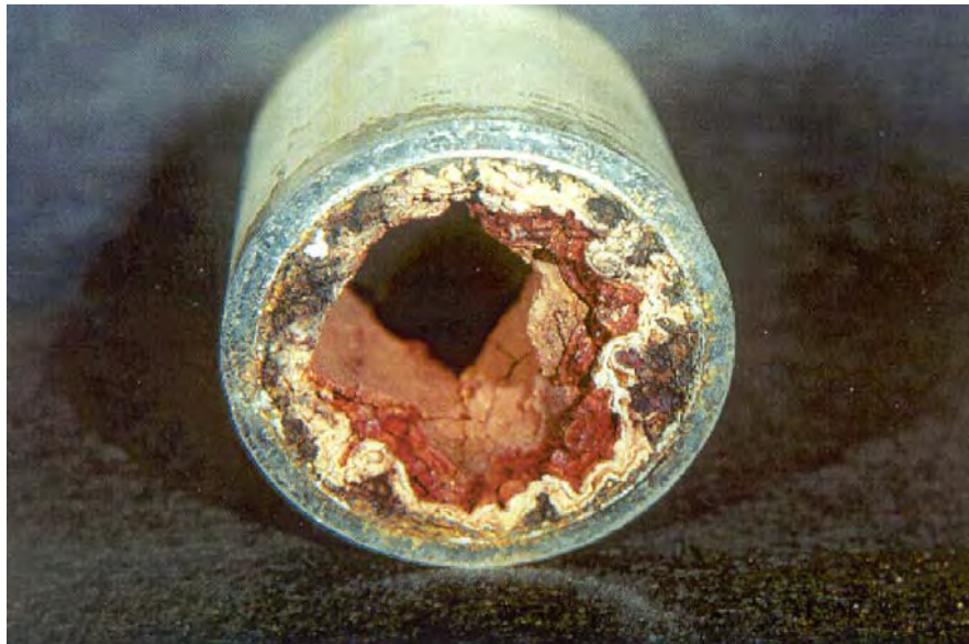
FIGURE 3-5. Scaled Boiler Tube
