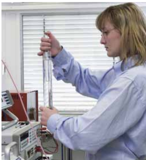
Fig. 16: Calibration with the water triple point cell
