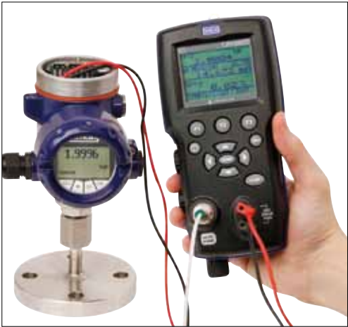
Fig. 26: Calibration of a pro- cess transmitter with portable calibrator
