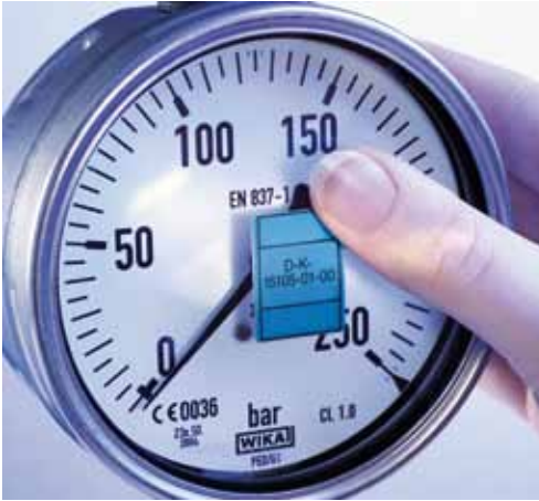
Fig. 6: Calibration sticker on a mechanical pressure gauge
