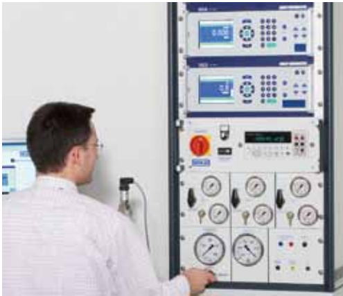
Fig. 17: Automated calibration of pressure measuring instruments
