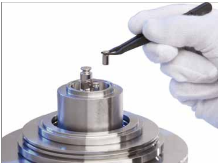
Fig. 13: Mass load, including trim masses of a few milligrams
