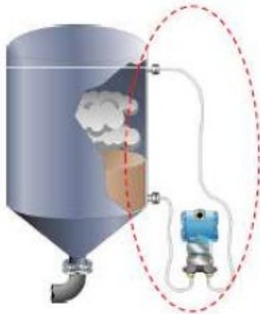
A circle representing locally mounted instrument
