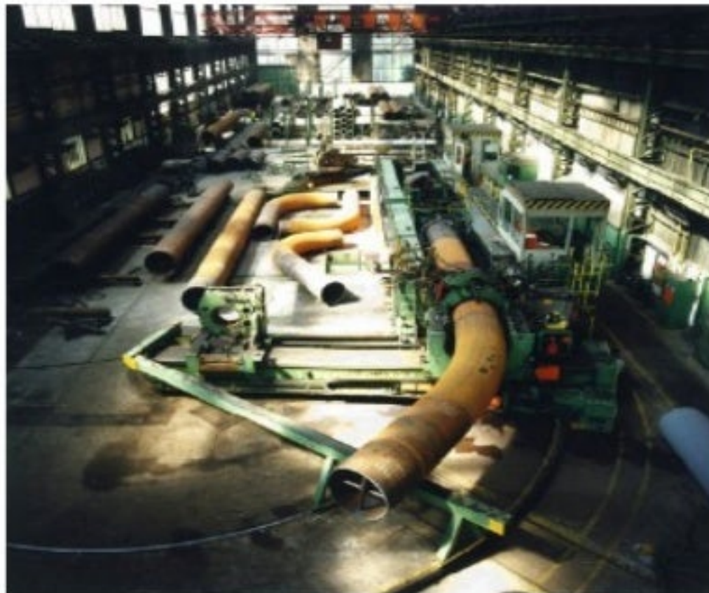
Figure 8: Hot induction bending of 48" line pipe at Mannesmann Bending Plant
