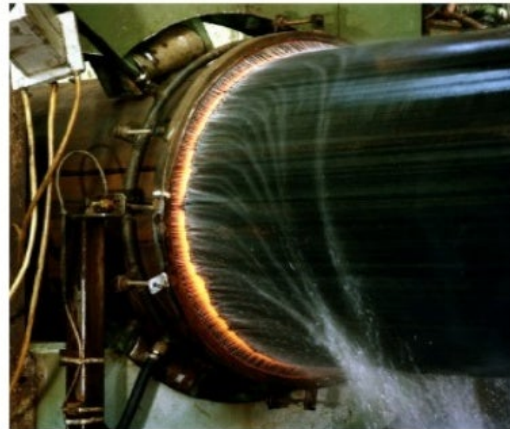
Figure 9: Detailed view on induction coil and heated zone during bending
