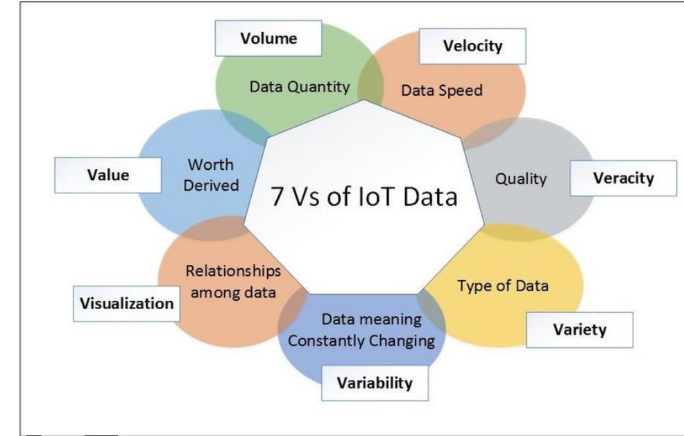
The **Internet of Things**, or **IoT**, is a system of interrelated computing devices, mechanical and digital machines, objects, animals or people that are provided with unique identifiers (UIDs) and the ability to transfer data over a network without requiring human-to-human or human-to-computer interaction.
