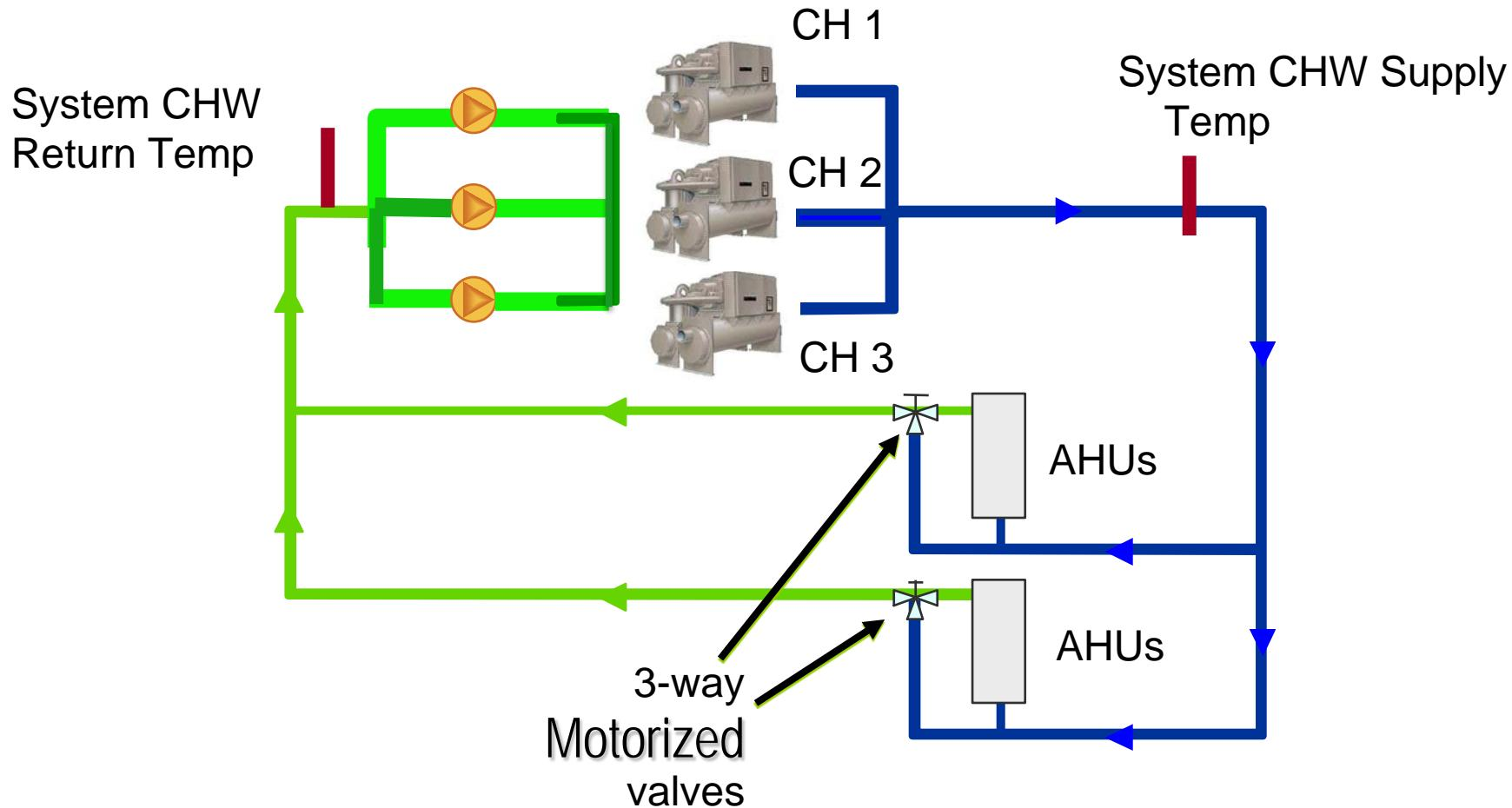
**Don't switch off pumps even if chiller one/two chillers are off**
