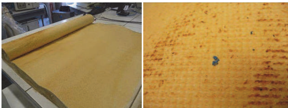
Fig. 8. Iron deposit on RO membrane
