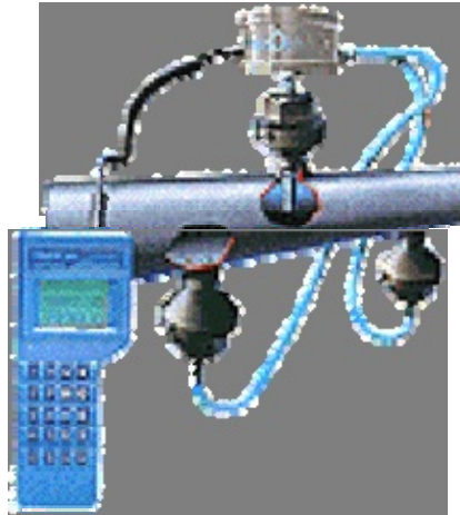
Electric measurement of corrosion (doc. Metal Samples)
