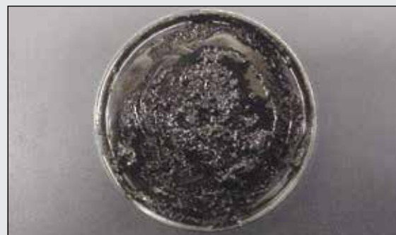
Fig. 65. This petri dish above contains heavily oxidized grease, which purged from an overfilled bearing. Grease undergoing heavy oxidation often has a very distinguishable black color and burned odor. In addition, it gets stiffer in consistency.
