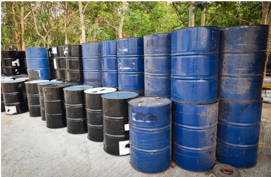
Figure 4-1: Drums stored with inadequate labelling and without secondary containment and sufficient fire breaks in the row
