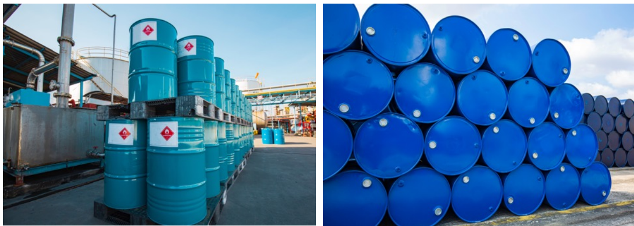
Figure 4-4 Left: Acceptable drum storage at correct height – two drums high and supported by pallets. Right: Unacceptable drum storage – drums stored on side, four high and requiring many drums to be removed to gain access
