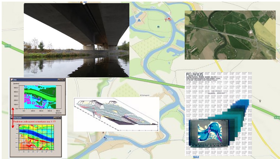
Figure 5.2 Highway bridge over the Ohre River close to Doksany, where the 2D model was used for the analysis of the position of the embankment of the designed bridge – first analysis in Central Europe using FLUVIUS 2D hydrodynamic unsteady model – results compared with scale air model (courtesy of DHI).
