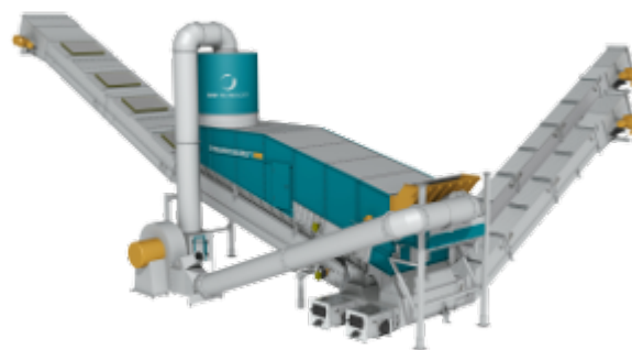
Figure 6-11: Air density separator example.
