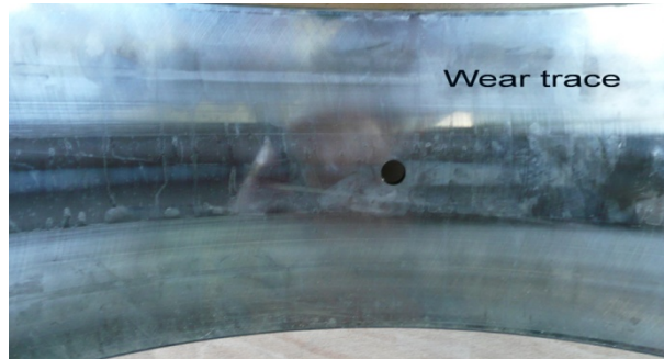
Abrasive wear on outer ring raceway ( SRB).
