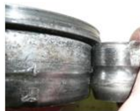
Well-worn rollers and raceway.
