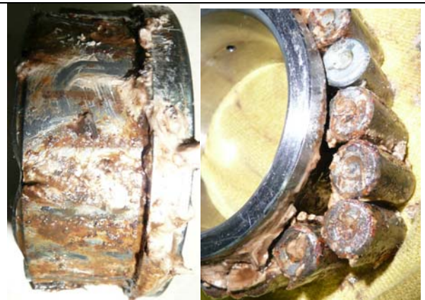
Corrosion. Contaminated lubricant.
