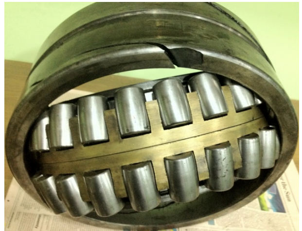
Outer ring crack. Fretting corrosion.
