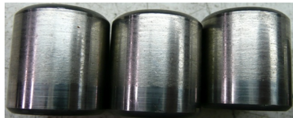
Length uneven running pattern on rollers
