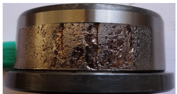
Even exfoliation on loaded area. Normal wear pattern.
