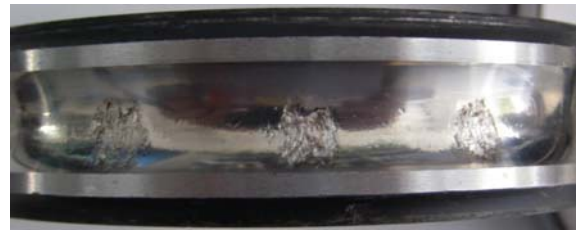
Spalling in the true brinelled areas due to mounting.
