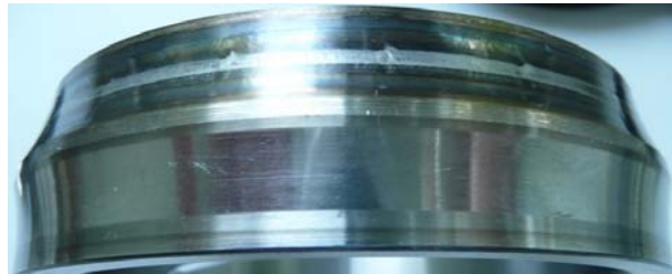
Uneven running pattern of inner ring raceway.
