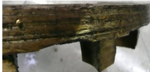
Worn cage pockets and seizure of outer surface
