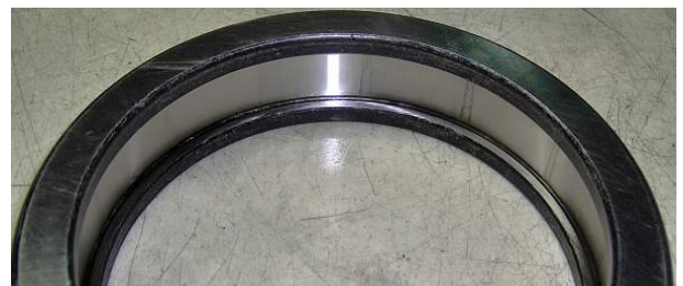
Corrosion while storage.
