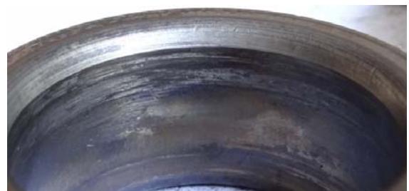
Smearing, polished surface of outer ring, fretting corrosion on inner ring bore
