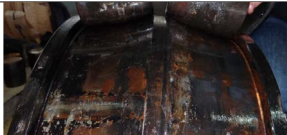
Advanced wear of raceways.
