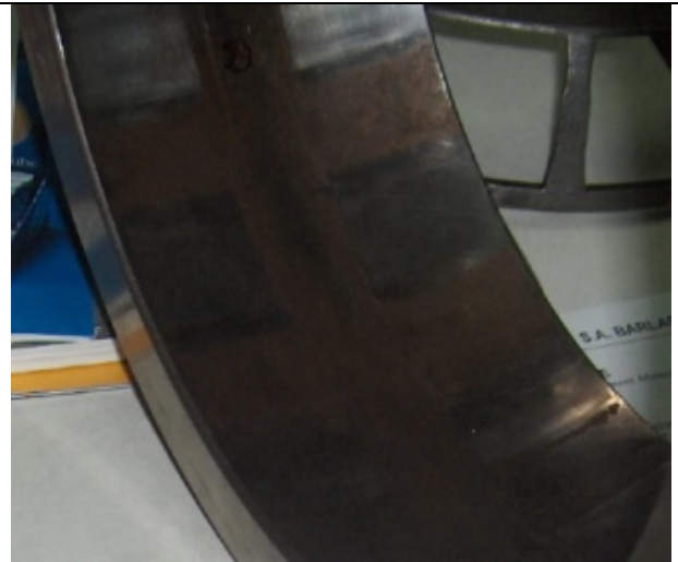
Corrosion while stationary.
