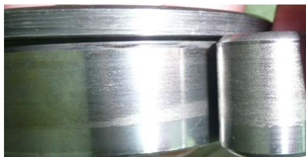
Smearing on inner ring raceway and roller
