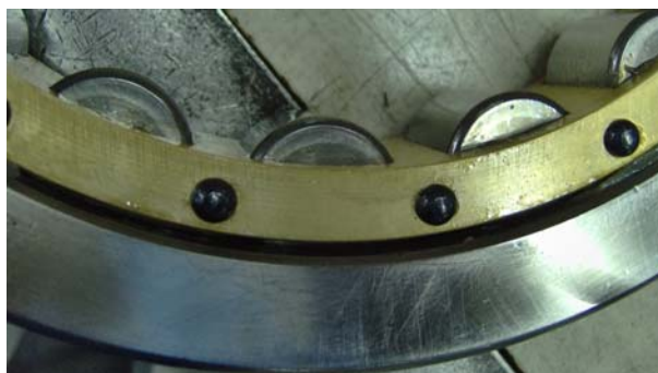
Wear on rollers end face of Cylindrical Roller Bearing.
