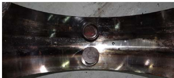
Advanced wear of one rollers row and for one part of outer ring raceway.
