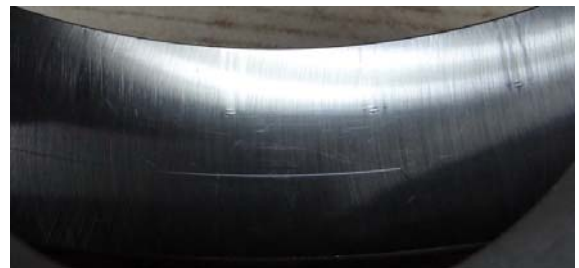
Raceway true brinelling – Spherical roller bearing
