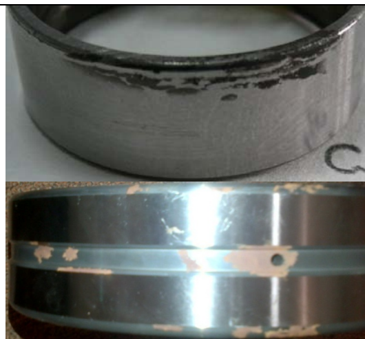
Front and outer corrosion on the outer ring
