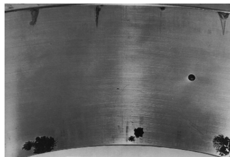
Corrosion in storage. The corrosion takes place underneath the rollers where moisture is trapped.
