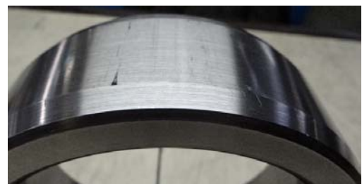
Raceway true brinelling – Cylindrical roller bearing
