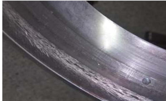
Uneven running pattern – half raceway scoring
