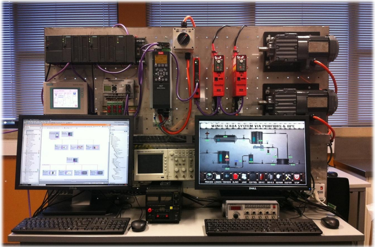
Figure 63: Portable project panel for testing and device configurations
