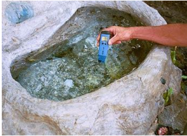
Testing a spring for electrical conductivity/ Total dissolved solids.
