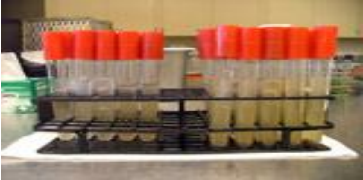
A-1 broth inoculation tubes from a multiple tube fermentation analysis for fecal coliform density.
