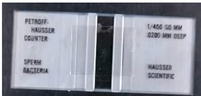
Figure 4-10 The Petroff-Hauser counting chamber
