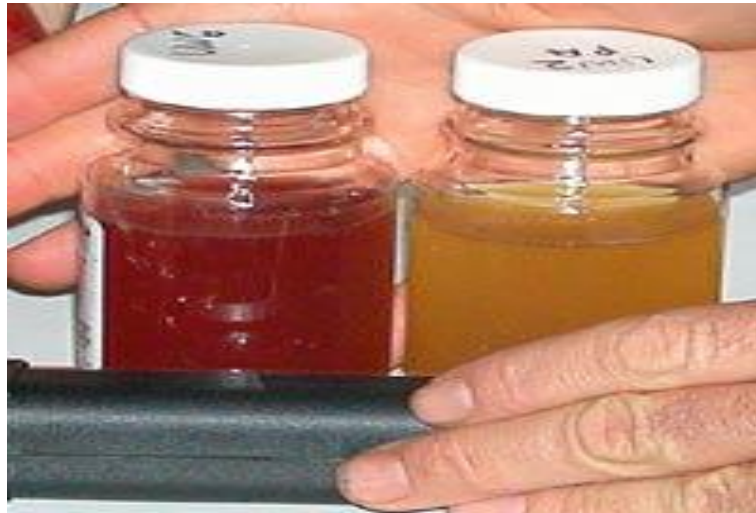
Tap water on right has no general coliforms. Same water after passing through a reverse/ osmosis drinking water filter (left) is positive for general coliforms. It's about to be tested with a UV light to see if it also has fecal coliforms (it didn't).
