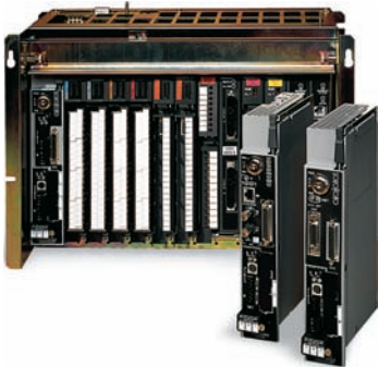
Figure 2-4 Allen-Bradley PLC-5 rack/slot-based addressing format. Source: Image Used with Permission of Rockwell Automation, Inc.
