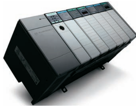
Figure 2-5 Allen-Bradley SLC 500 rack/slot-based addressing format. Source: Image Used with Permission of Rockwell Automation, Inc.
