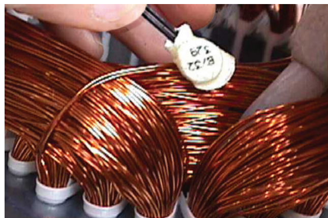
Figure 7.6 - Thermostat installation in the winding
