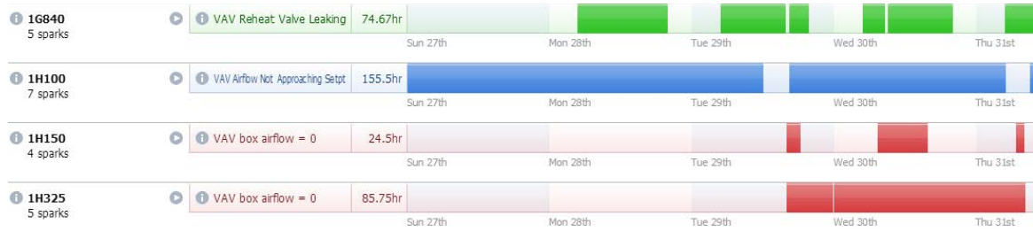
Figure 17. Zone-level fault detection and diagnostics
