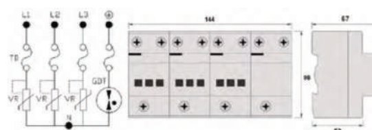
Electrical diagram and dimensions of BD4-60
