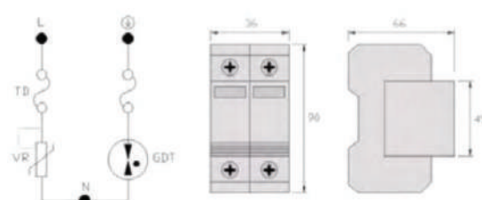
Electrical diagram and dimensions of BD2-20
