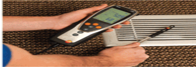
Recognized testing and balancing methods include, clockwise from top: circuitry checks, air velocity readings, and flowhood testing. PHOTOS COURTESY NATIONAL COMFORT INSTITUTE
