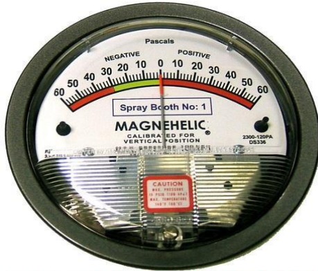
MAGNEHELIC DIFFERENTIAL PRESSURE GAUGE
