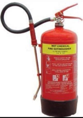
Portable Wet Chemical extinguishers are used for cooking oil / fat fires. The fine spray gives almost immediate flame extinguishment while the wet chemical agent reacts with oil to form a soap-like film to seal the surface of the oil and cool it down to prevent re-ignition.
