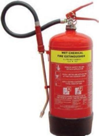
Portable Wet Chemical extinguishers are used for cooking oil / fat fires. The fine spray gives almost immediate flame extinguishment while the wet chemical agent reacts with oil to form a soap-like film to seal the surface of the oil and cool it down to prevent re-ignition.
