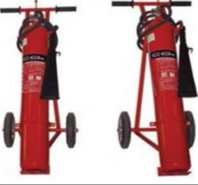
Portable Carbon Dioxide Fire Extinguishers are known for its high reliable performance and ease of handling. The cylinder for CO<sub>2</sub> Fire Extinguishers are seamless and extruded from high grade Chrome Molybdenum Steel or Manganese Steel or Carbon Steel. Carbon Dioxide is discharged as a white cloud of snow which throttles a fire by eliminating the oxygen. Designed to protect areas where class B (flammable liquids and gases) or Electrical class of fires could occur.
