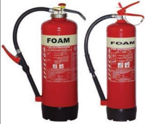
Portable Foam Fire Extinguishers are characterized for their quick fire suppression and extinguishing capabilities, especially oil, petrol and other liquid fire. It works by covering a burning flammable liquid with a blanket of foam, cutting off the fire's air supply and preventing the release of flammable vapours. Portable foam extinguishers are generally used as first attack fire fighting units which are suitable for class A and B fires.
