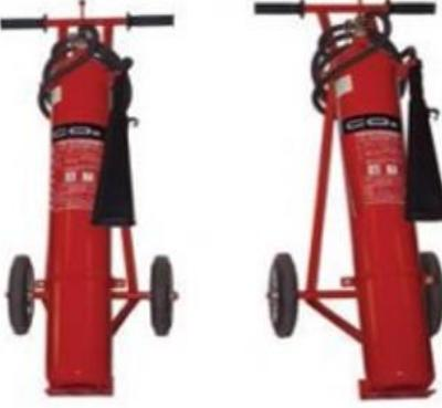
Portable Carbon Dioxide Fire Extinguishers are known for its high reliable performance and ease of handling. The cylinder for CO2 Fire Extinguishers are seamless and extruded from high grade Chrome Molybdenum Steel or Manganese Steel or Carbon Steel. Carbon Dioxide is discharged as a white cloud of snow which throttles a fire by eliminating the oxygen. Designed to protect areas where class B (flammable liquids and gases) or Electrical class of fires could occur.
