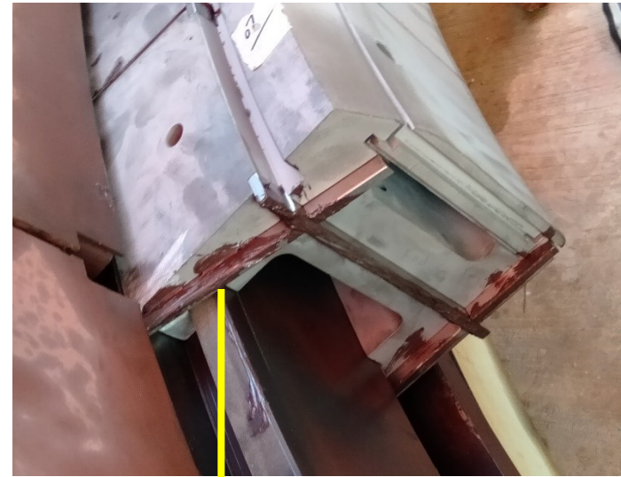
Cloth Seal Arrangement b/w 1 st stage shrouds
