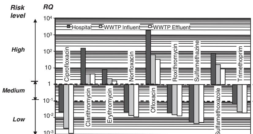
Fig. 2. Risk quotients for antibiotics in Hospital B effluent and investigated WWTP influent and effluent.
