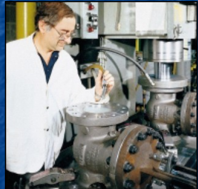
After assembly, pressure testing of shell, seats, packing and backseat to API 598.
