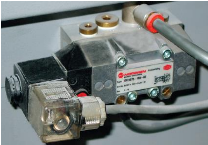
Pilot operated solenoid used to switch the flow of air
