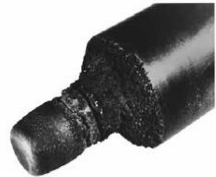
Typical Appearance of Cavitation Damage
