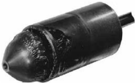
Typical Appearance of Flashing Damage
