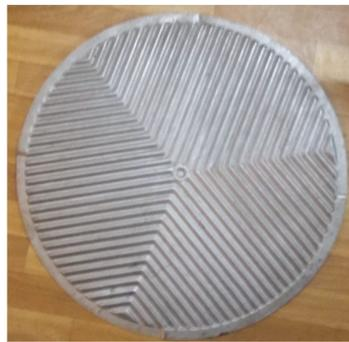
**Figure 1.** The plate of WPHE for an ammonia synthesis column.
