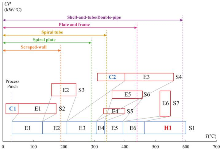
Figure 7. SRTGD-STR of the existing HEN for the case study.
