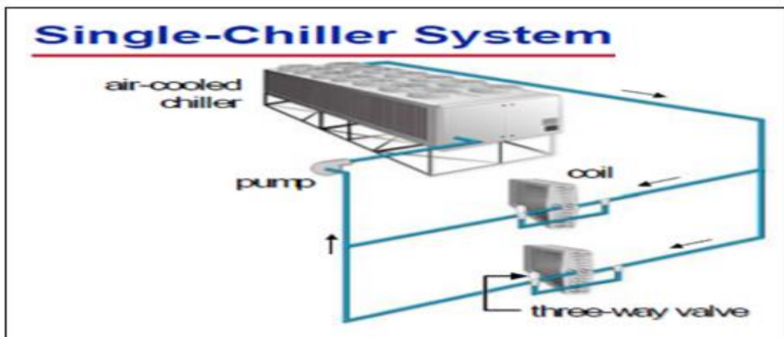
Fig (31).single chiller system
