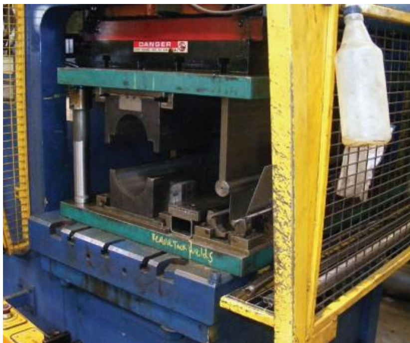
Figure 1: This 175-ton hydraulic press was severely damaged by lightning, necessitating repair or replacement of many key components, including the automation system.
