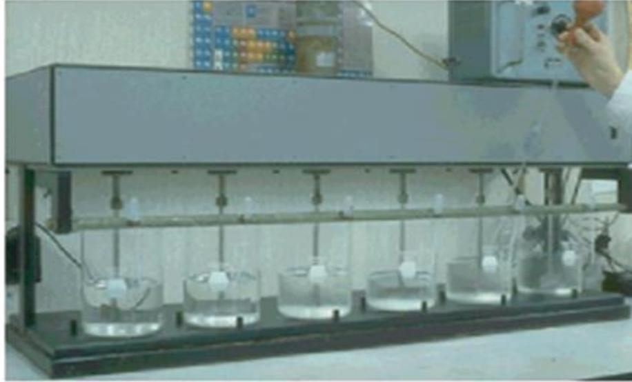
Figure 9 - Jar-test apparatus
