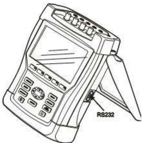
Tilt stand and location of RS-232 interface
