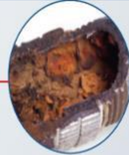
Galvanic Corrosion in the Presence of an Electrolyte
