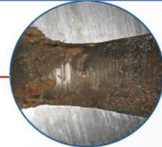
Sour Gas Cracking or Sulfide Stress Cracking at High Hydrogen Sulfide (H 2 S) Partial Pressure
