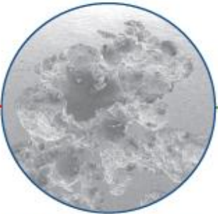
Localized Pitting Corrosion in Chloride-Containing Media
