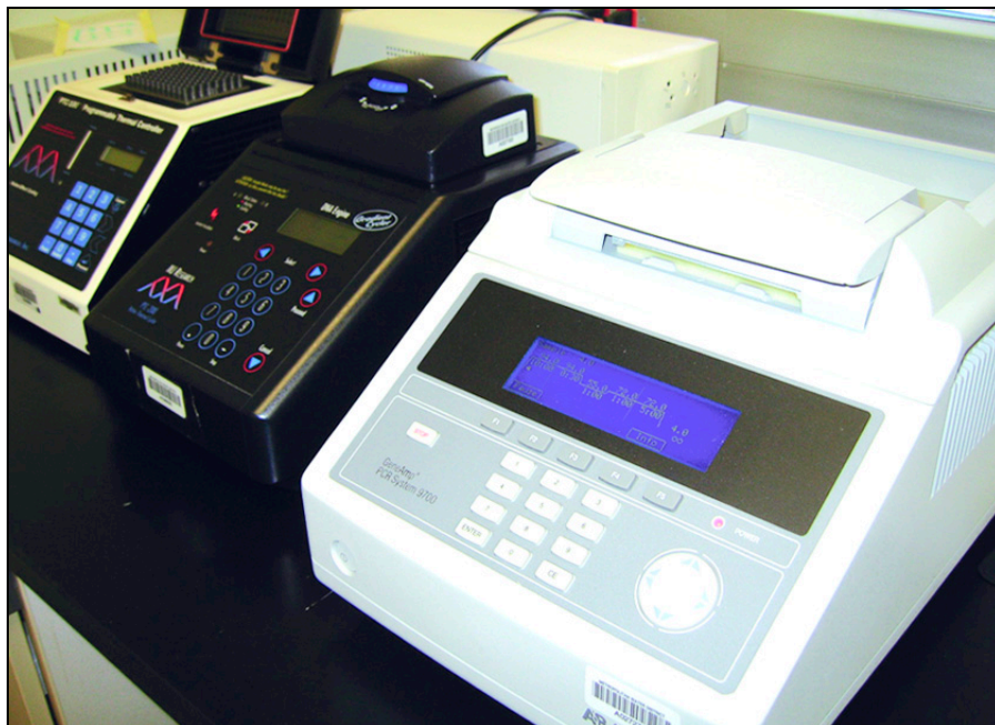
Figure 4-3 Thermal cyclers used to automate the temperature cycling steps of polymerase chain reactions
