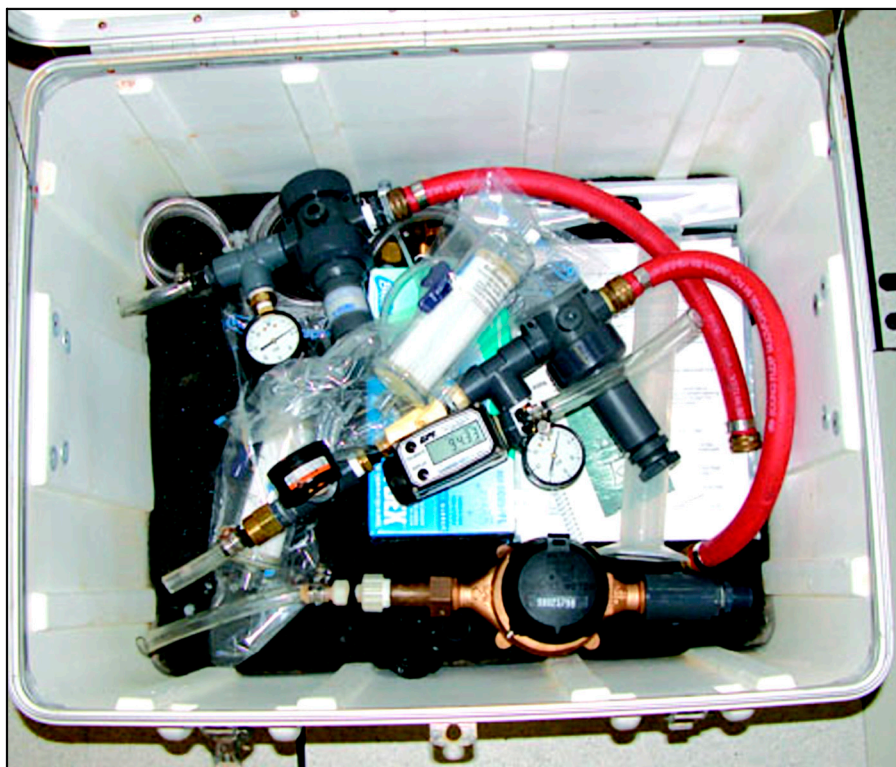
Figure 3-6 Pathogen sample kit. Various types of hoses, connectors, and dechlorination equipment can be stored and ready for use.
