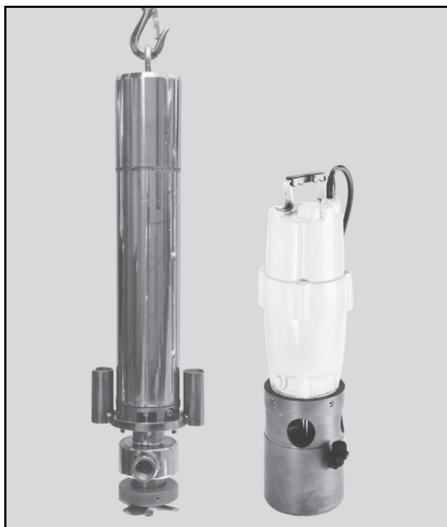
Figure 4-14 Chemical induction mixers use a high-speed impeller to create a vacuum to draw the chemical, gas, or liquid into intimate contact with water to be treated. Some mixers have an open impeller design (left) and some are closed (right).
