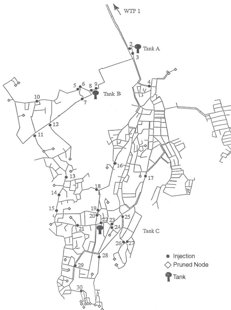
Figure 6-8 Network map with potential booster chlorination locations
