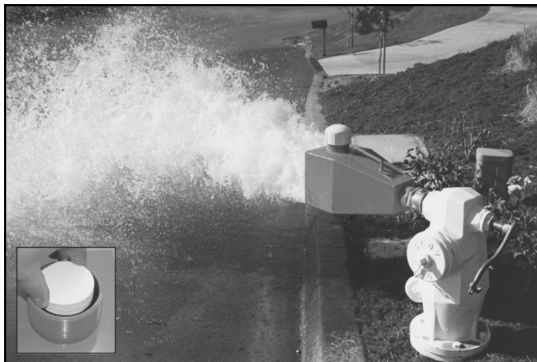
Figure A-3 Diffuser for dechlorination of hydrant or blowoff waters
