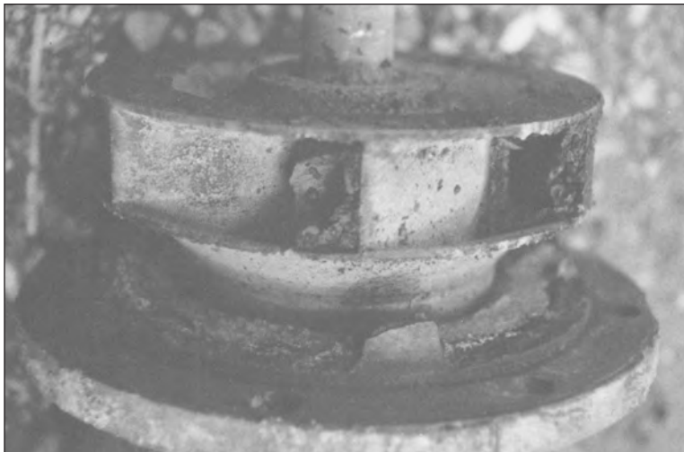
Figure 2-6 Partly filled impeller channel
