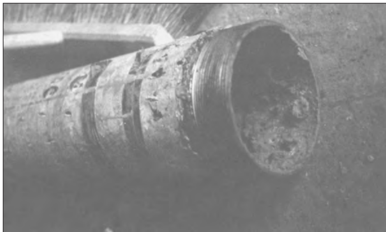
Figure 2-8 Column pipe with iron biofilm
