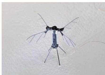
Figure 9. Miniature robot with insect-like flight capabilities, [119].
