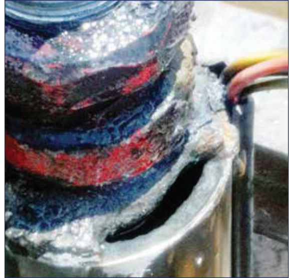
FIGURE 5.10 Stray electrical currents formed a hole in this submersible pump, causing the well to fail.
