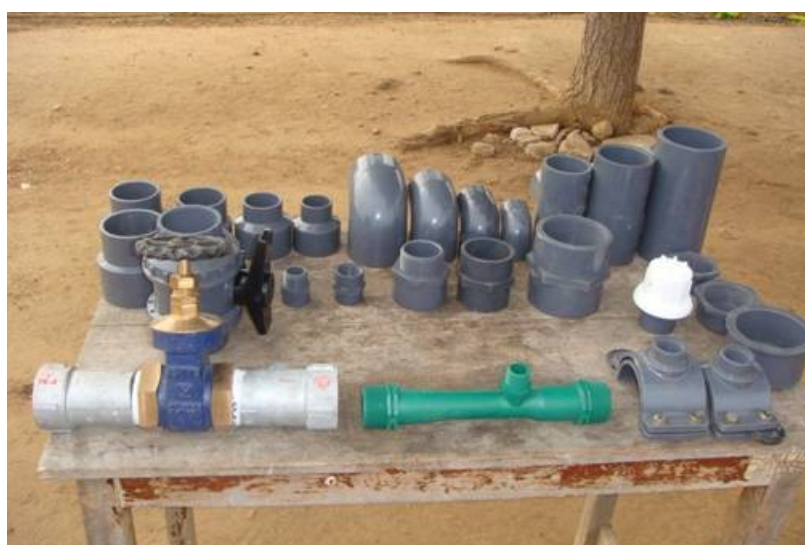
Figure 1-12: Drip irrigation valves and differentPVC fittings
