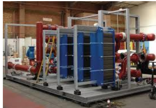
Figure 155: plate heat exchanger installation
