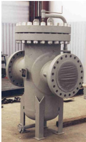
(a) Inlet and Outlet on Opposite Sides
