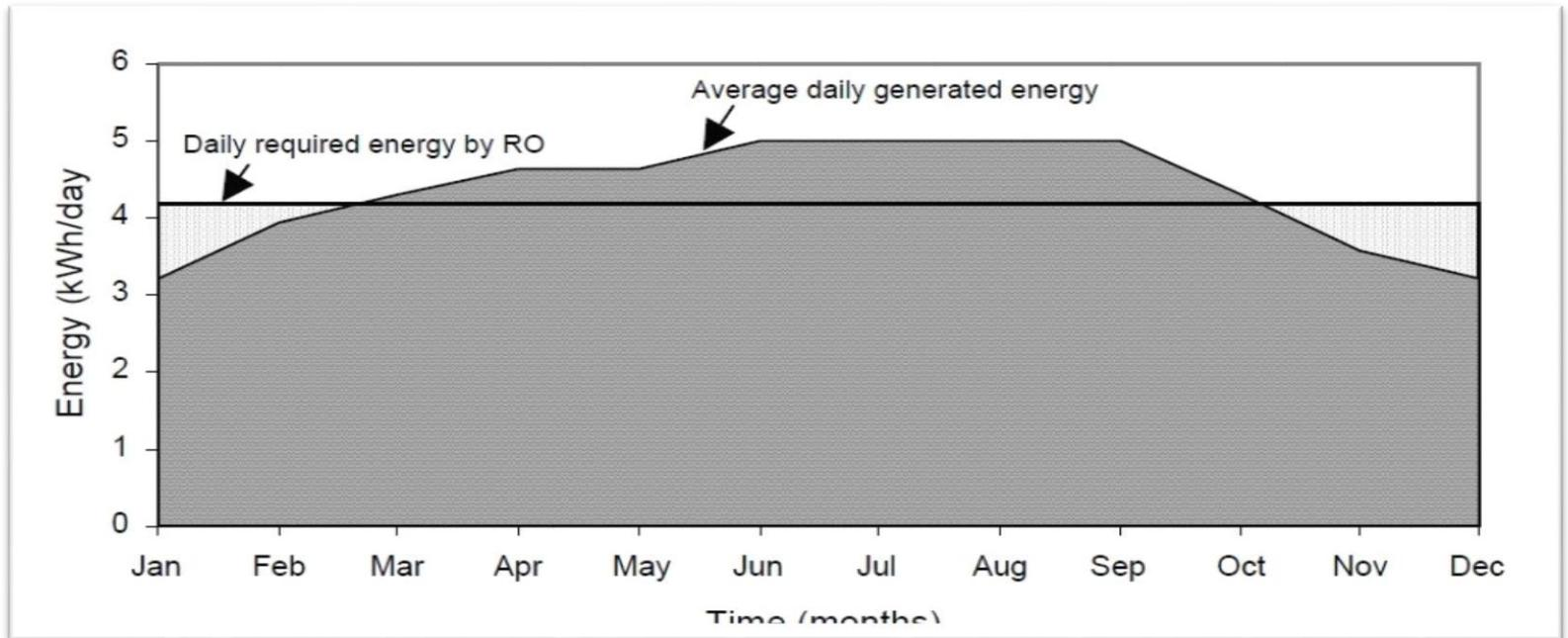
Figure 3 The average daily generated energy versus that required by the RO unit at different months
