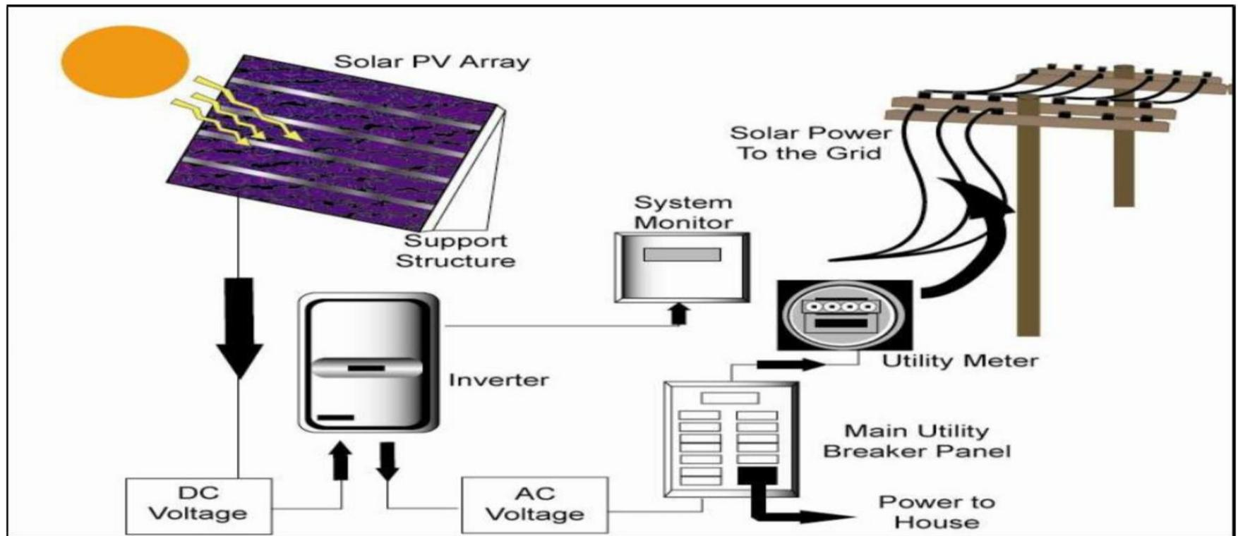
**Grid-Tied PV System (ON-GRID)**
