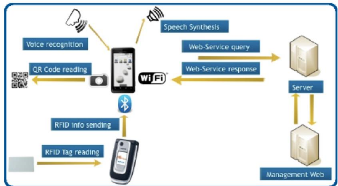
QR coding enhanced by RFID tagging architecture
