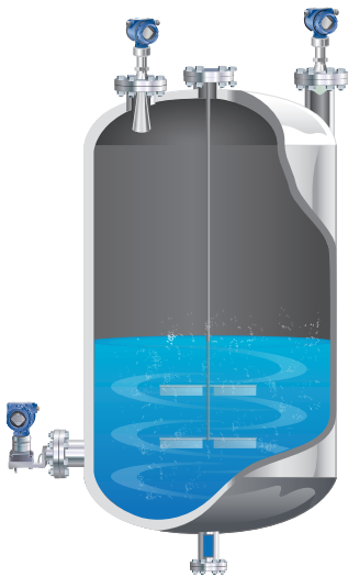
Figure 4.8.1: Level measurement in a tank with agitation
