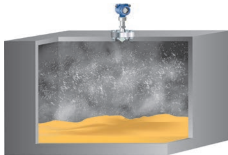
Figure 4.10.1: Rosemount 5408 process seal with nozzle installation
