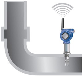
Figure 4.18.5: A wireless with detecting wether there is liquid or not in the pipe
