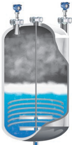
Figure 4.9.1: Reactor vessel level with non-contacting radar
