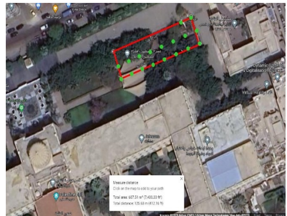
Figure 73: Borehole field configuration [For Acoustics Building]
