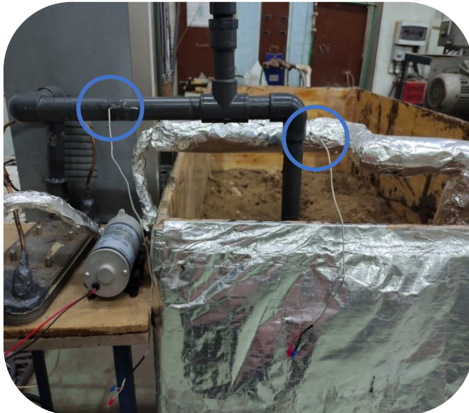
Figure 25: Sensors at various points of the prototype
