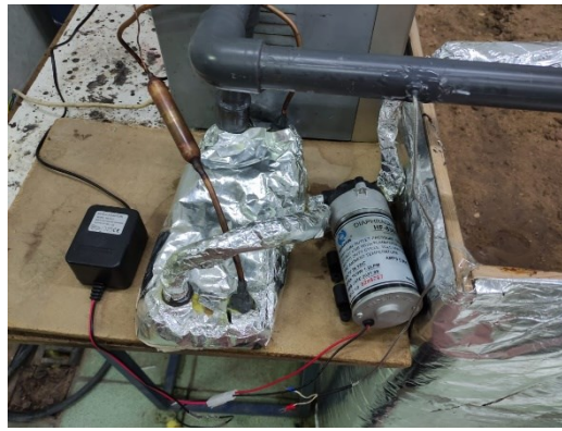
b) plate heat exchanger + diaphragm pump
