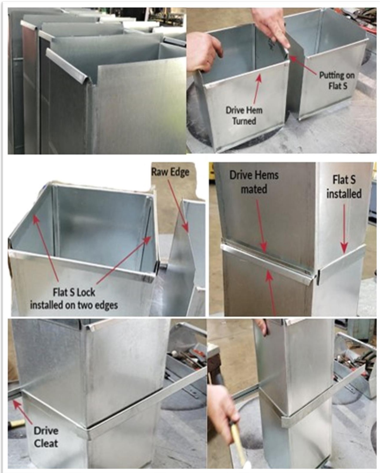
Slip and Drive Ducting Connection method
