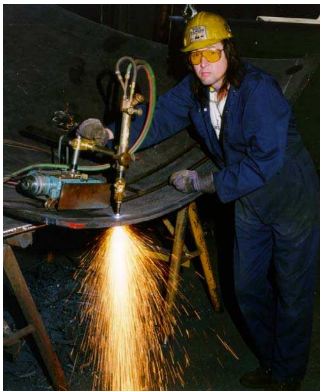
Figure 4.1 An oxygen cutting torch is used to cut the shaped plate to length. After cutting, the slag and metal discoloration will have to be mechanically removed (UG–76).
