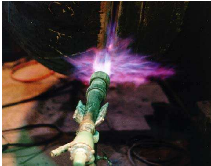
Figure 4.12 A torch is used to preheat this thick walled material prior to making the shell-to-head weld.
